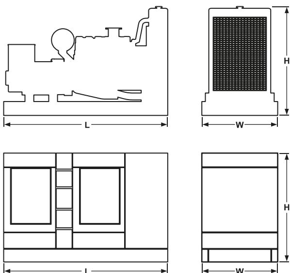
Dimensions in centimeters, dry weight, do not use for installation design. See general dimension drawings for detail. Please contact the department of engineering for exact dimensions and weight.
